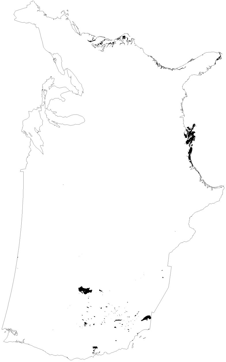
Figure B-5: Approximate areas that may have frequently flooded in the past (e.g., dry lake beds, salt flats, areas below sea level). Proposed sites located in these areas may require additional site characterization and analysis (ESRI, 2008a; ESRI, 2008b)
